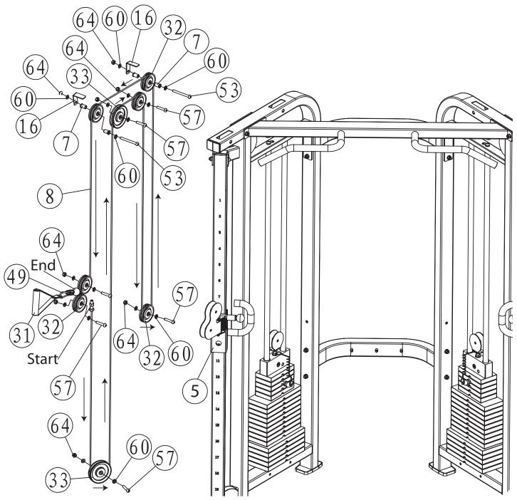
STEP 5 Start by threading one end of the Pulley Cable (8) into Left Slip Frame (5). Remove hardware and ball from the other end of the cable. Follow the diagram above to complete the cable installation. Note: When installing the cable, make sure the cable is centered on the pulley and is not rubbing against any part of the frame or any hardware.
